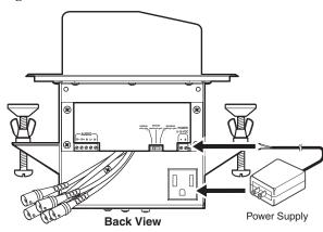
Figure 2-10 — Powering the Extender board
